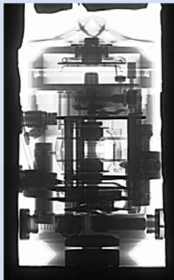
339 Cluster Munition Fuse Mechanism (X-ray with Seifert Eresco MF2 Continuous Industrial Source – Exposure 4 seconds, with foX-Rayzor)
