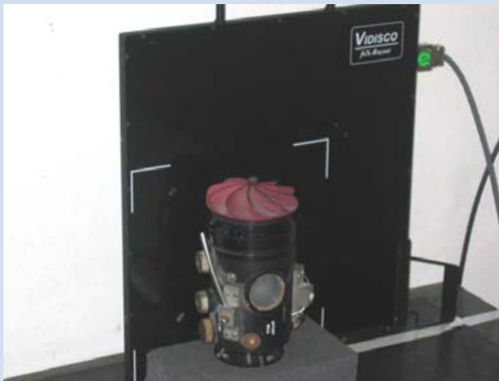
339 Cluster Munition Fuse Mechanism (X-ray with Seifert Eresco MF2 Continuous Industrial Source – Exposure 4 seconds, with foX-Rayzor)
