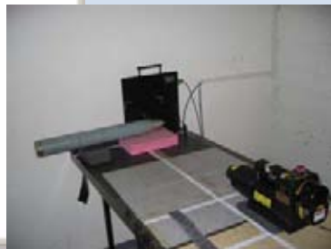
EW Electronic Warfare Rocket Head X-ray, Taken with foX-Rayzor and XRS-3, 65 Pulses
