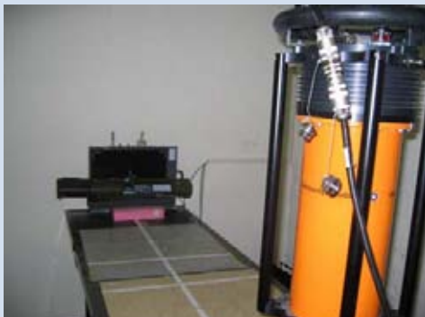
RPG 22 Munition Inspected with Flat foX-17 and Seifert Industrial Continuous Source
